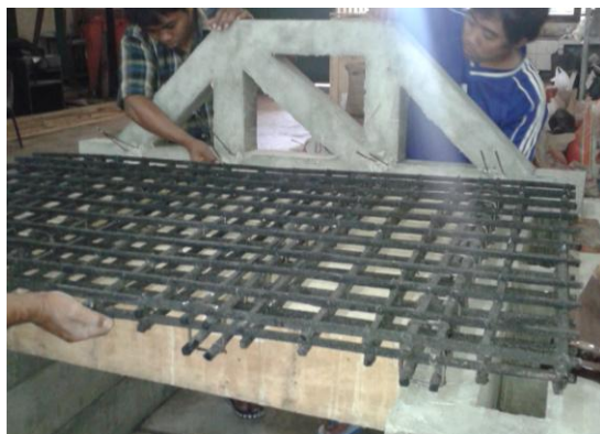
Figure 6 The slab reinforcement
