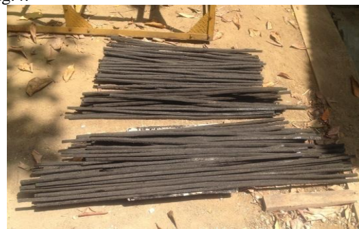
Figure 4 The bamboo reinforcement
