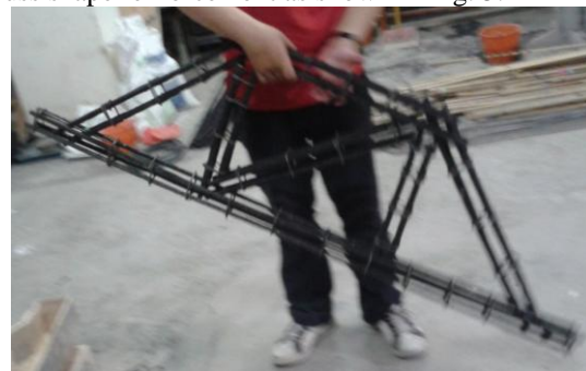
Figure 5 The truss reinforcement
